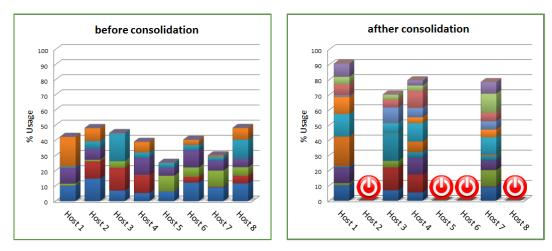
Figure 2 – Example of servers usage before consolidation (left) and after consolidation (right). In this simple case consolidation allows half servers to be hibernated.
