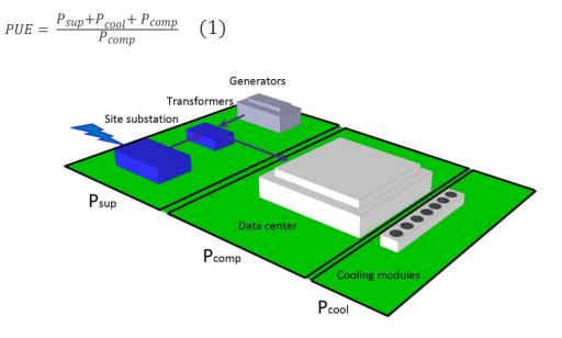
Figure 1 – Power usage in a data center
