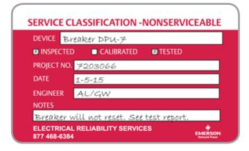
Figure 1. Field testing labels help satisfy documentation requirements of NFPA 70E 2015.
