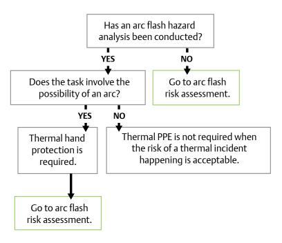
Figure 2. The thermal risk assessment process for a battery system illustrates how the likely exposure depends on the type of task being performed.
